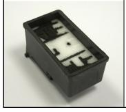
By milling the cap and inserting a sponge PartNo. 4010 0305, cartridge PG-510/545 will reach same capacity as PG-512/545XL.
