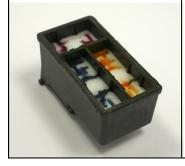
By milling the cap and inserting sponges PartNo. 4010 0406 & 4010 0307, cartridge CL-511/546 will reach same capacity as CL-513/546XL.
